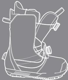
When putting on or removing the boot, pull the reel out to release tension, then pull the tongue forward and push in the reel to lock it in place.
